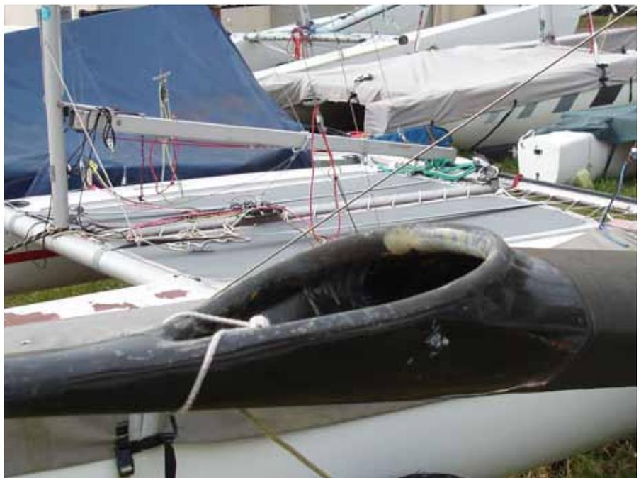
The spinnaker chute edge suffers from rope burns. This can be protected by a PSP Anti Chafe patch, which also reduces friction, allowing the spinnaker to be launched and recovered more easily.
